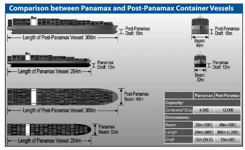
Comparison between the largest Panamax container vessel that can transit the current Canal and a Post-Panamax size vessel with 12,000 TEU's container capacity. The larger vessel has 2.5 times the cargo carrying capacity of the Panamax vessel.
